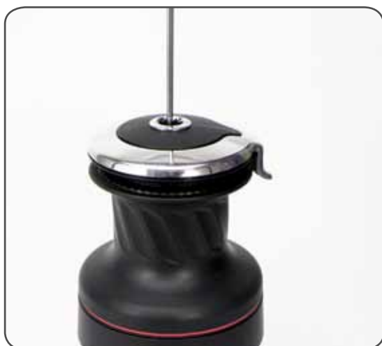
1. Unscrew the central screw ( \approx 2\text{Nm}/18\text{ in-lb} )
