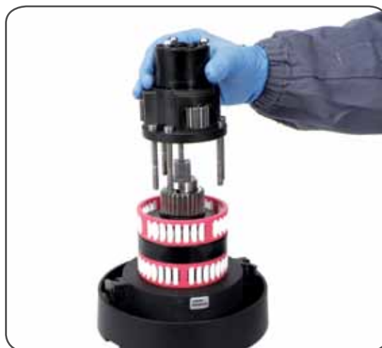
6. Slide off the gear carrier n°21. Pay attention to rollers in the gear carrier.
