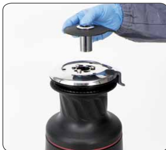
2. Slide off the assy socket n°31 and the cover n°13
