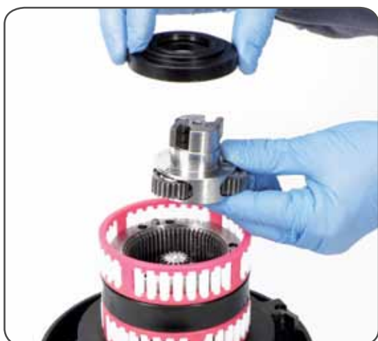
9. Remove the second planetary assy n°24 and remove flange n°11. Pay attention to the o-ring n°10 in the ring gear.
