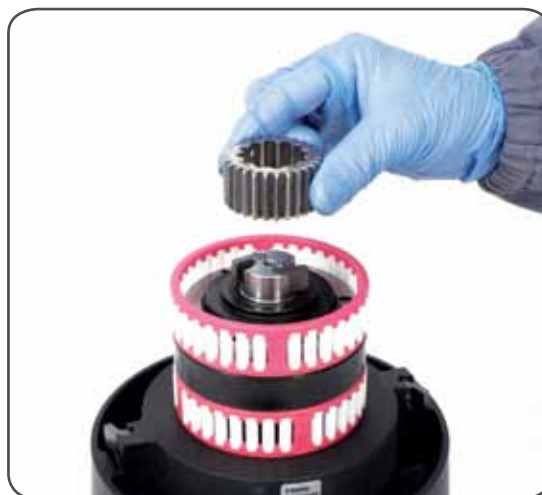
8. Lift off the gear n°9
