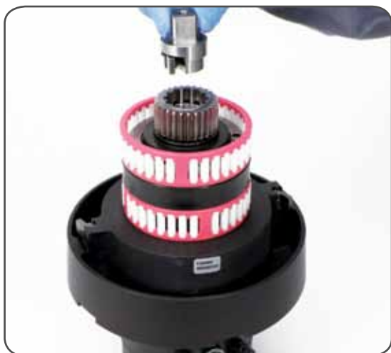
7. Slide out the pawls carrier n°20
