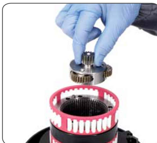
10. Slide out the first planetary assy n°23, the ring gear n°4, the o-ring n°10 and the pinion n°2.
