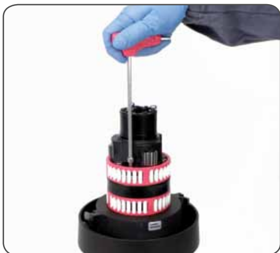
5. Unscrew the 6 hex screws n°18 (20Nm/177 in-lb)
