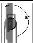
Block load increases when the line turns at a greater angle. Block loads double when the line turns 180°. If there is 400 kg (880 lb) on the line and the angle of deflection is 180°, the Harken through–deck block is subject to 800 kg (1760 lb). Select blocks carefully. See specification chart on next page.
