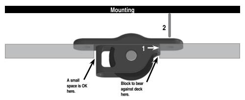
Refer to chart for fastener holes and choose appropriate drill size for through holes or tapping. **IMPORTANT!** When mounting the Protexit block:
