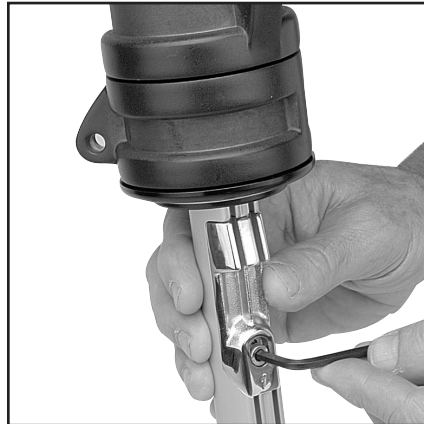
Loosen screw one revolution only.
