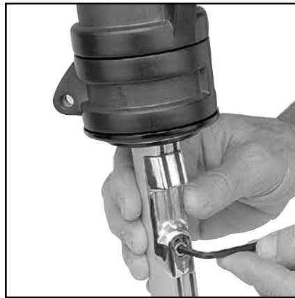
Loosen screw one revolution only .
