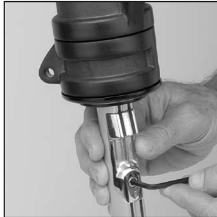
Loosen screw one revolution only .
