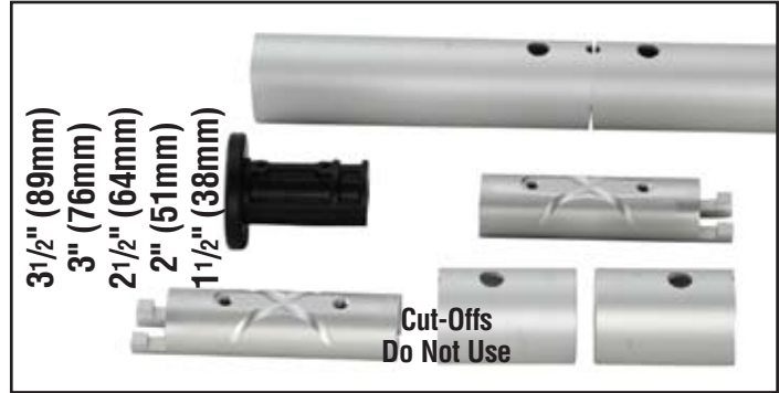
31/2" - 11/2" (89 - 38mm) Shorten top foil and adjoining full length foil so two screws are used to assemble joint instead of four. Do not use plastic bushings above top connector.
