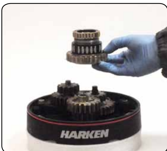
12. Remove the gear n°31, pawls carrier n°33, the bearings n°34 and 36 and the spring n°35
