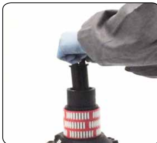
8. Slide out the assy clutch n°37
