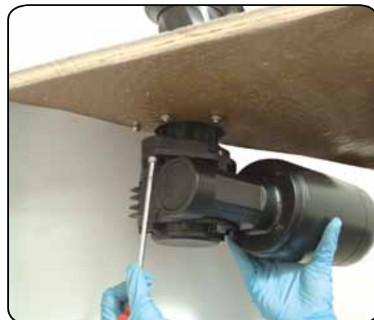
4. Tighten the two screws (8 Nm/ 71 in-lb). Be sure to align the flange.
