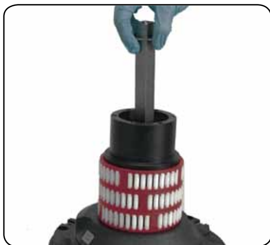
9. Slide out the central shaft n°19
