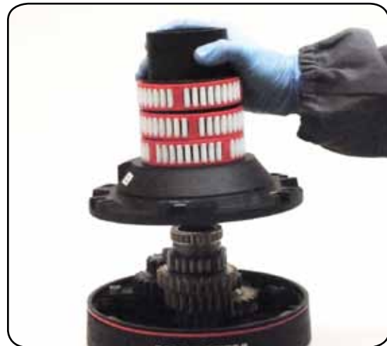
11. Slide out the drum support n°16
