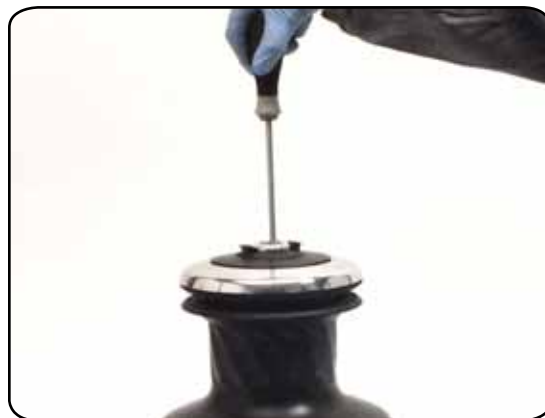
2. Unscrew the central screw ( \approx 2\text{Nm}/18\text{ in-lb} )
