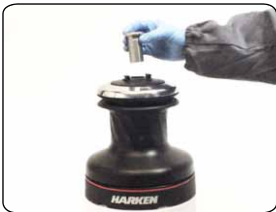
3. Slide off the assy socket n°30 and the cover n°29
