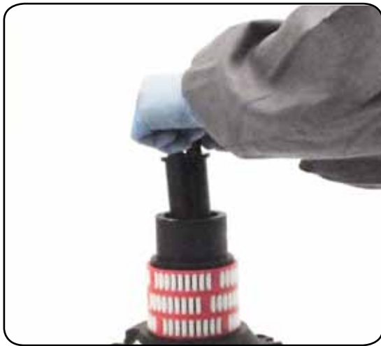
8. Slide out the assy clutch n°37
