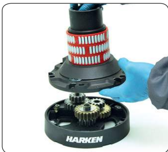
11. Remove the assy housing n°16
