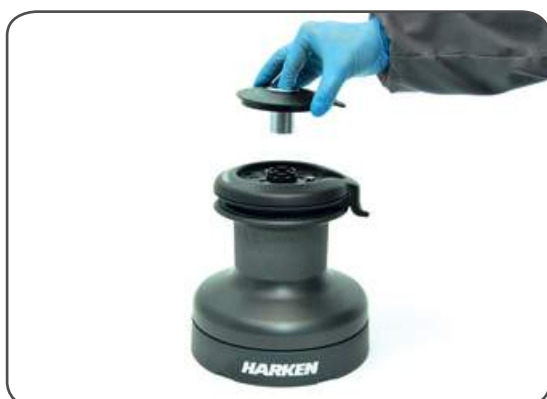
3. Slide off the assy socket n°29 and the cover n°28. Pay attention to the o-ring in the socket.
