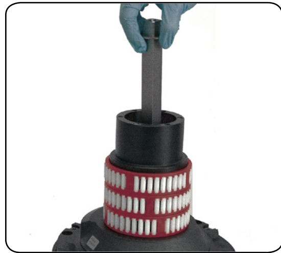
8. Slide out the central shaft n°19
