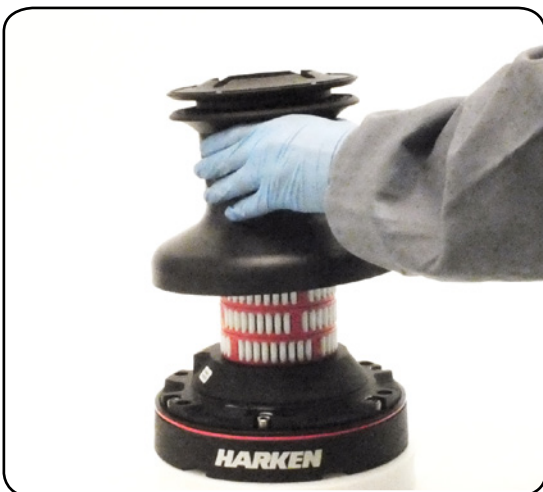
5. Lift off the drum n°24
