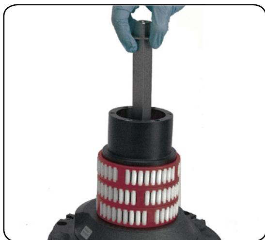
8. Slide out the central shaft n°19
