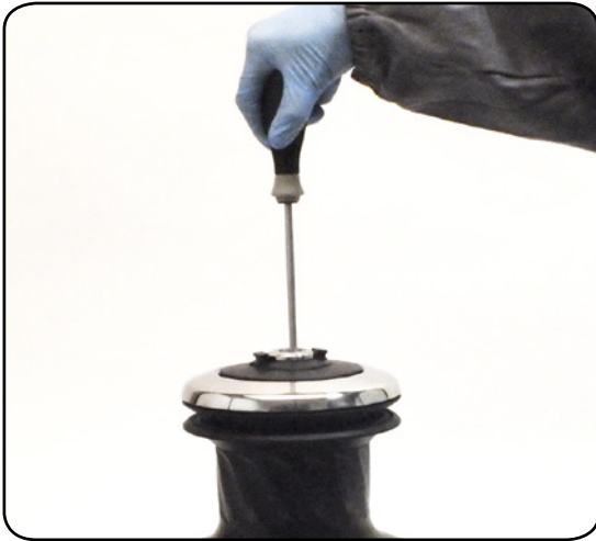
1. Unscrew the central screw (🔧 2Nm/18 in-lb)
