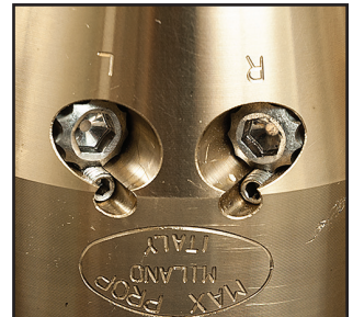
Fig.5 - Close up of the Left and Right pitch adjustment bolts.
