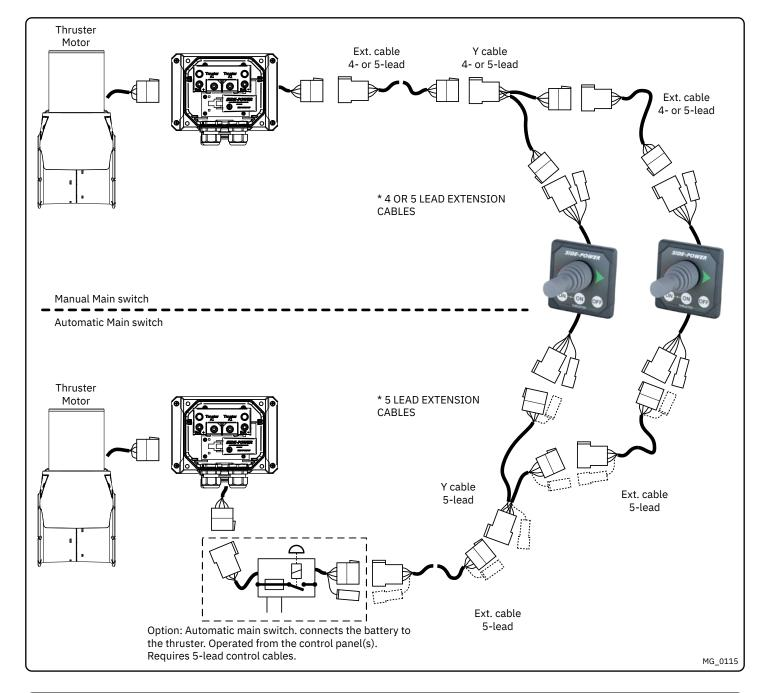
Control Panel Cable Installation MC\_0041
