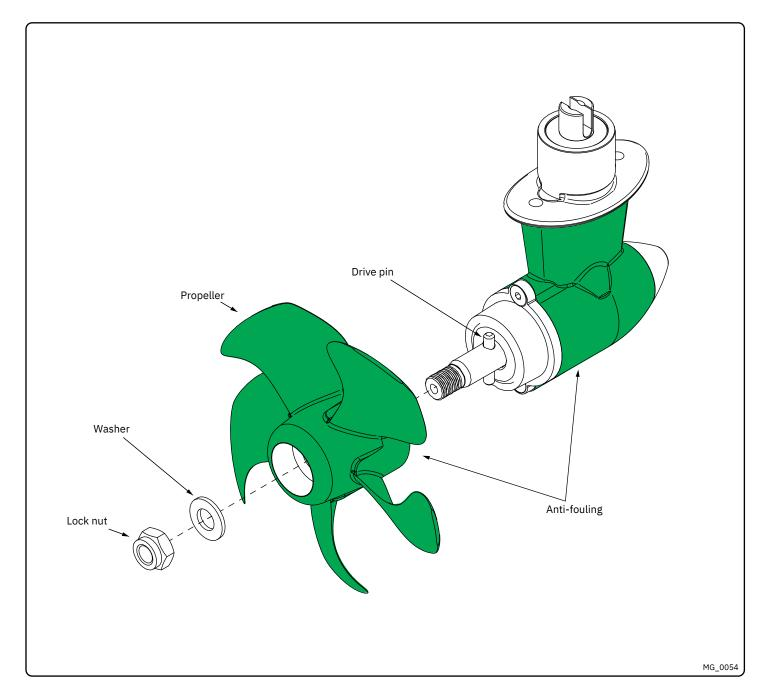
Propeller Installation MC\_0016
