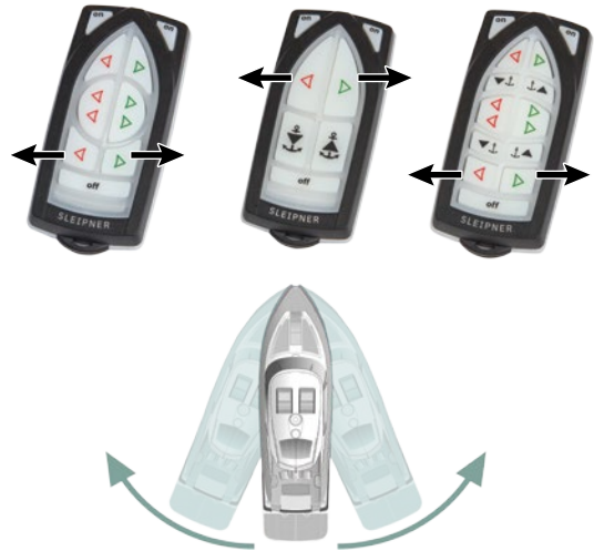
Activating the stern thruster
