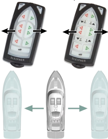
Activating both bow and stern thruster to push the boat sideways
