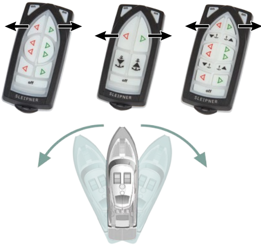
Activating the bow thruster
