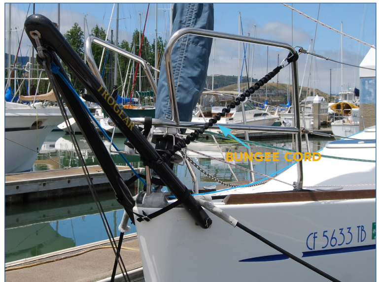
Fig 14: Showing Bungee Cord and Stop Strap.
