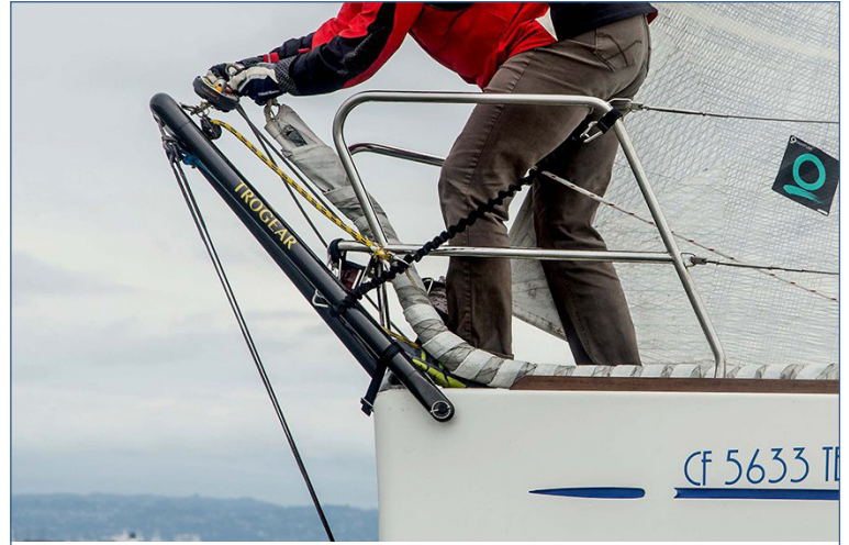
Fig 13: Bowsprit in upright position to attach a furler.
