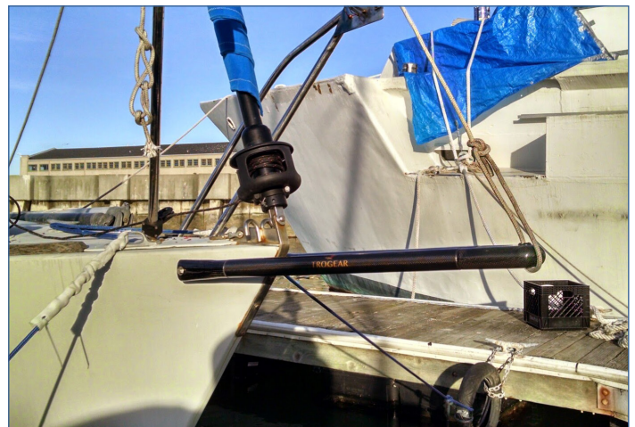
Fig 12: Temporarily secure the Bowsprit with a line
