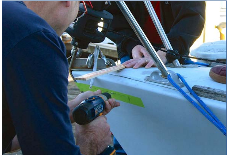
Fig 6: Drill a pilot hole first.
