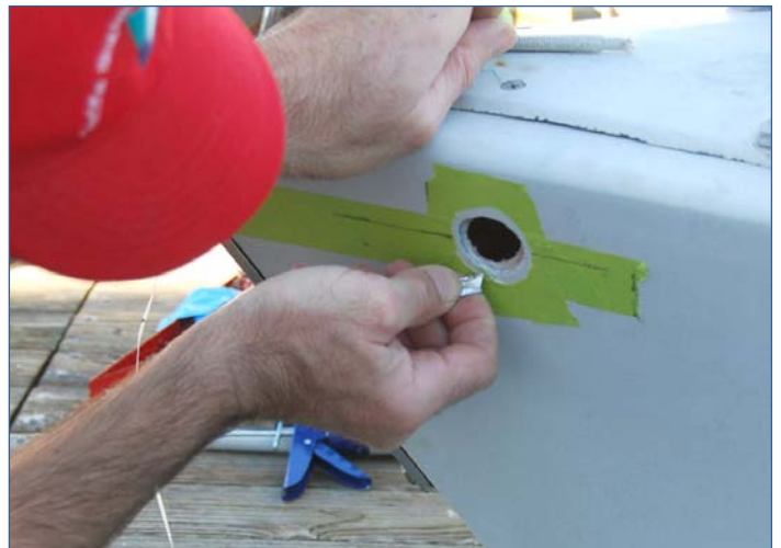
Fig 9: Leave about ¼ " exposed for epoxy fillet.
