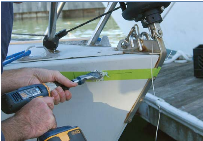
Fig 7: Drill holes using a 1" step drill.
