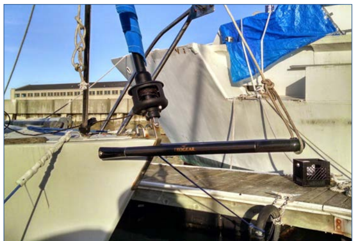
Fig 12: Temporarily secure the Bowsprit with a line
