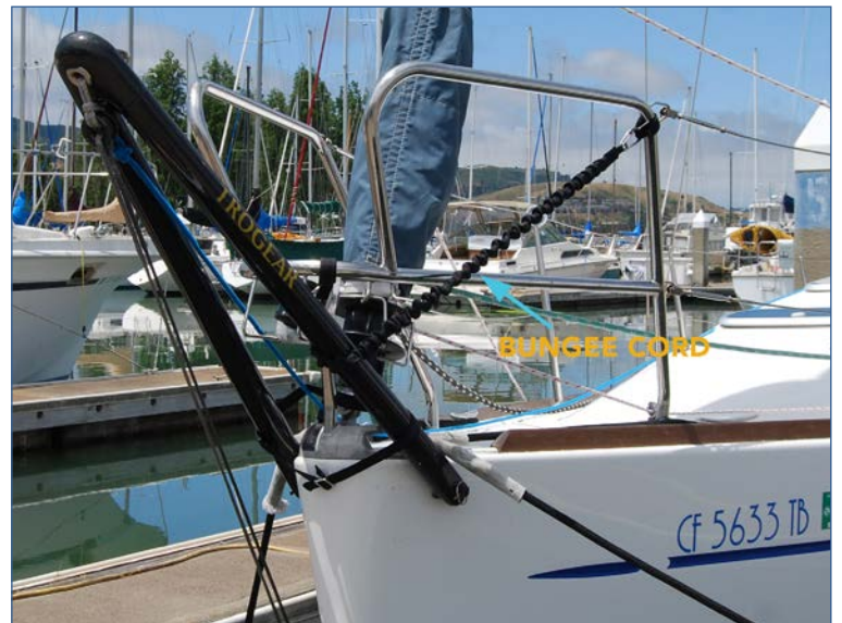
Fig 14: Showing Bungee Cord and Stop Strap.
